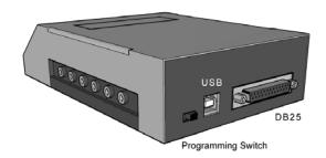
The X-keys USB Switch Interface has a DB25 connector on the back panel which serves as an alternative connection to the 12 ports. If both the ports and the DB25 connector are used, the switches are in parallel. If either switch is pressed, the programmed macro will be fired.
